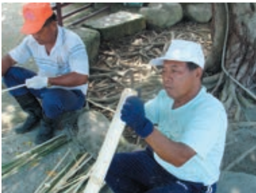
砍下的竹桿，先去節間小枝，再對剖成四大竹片。 Remove twigs from the cut cane then split it into four large parts.
