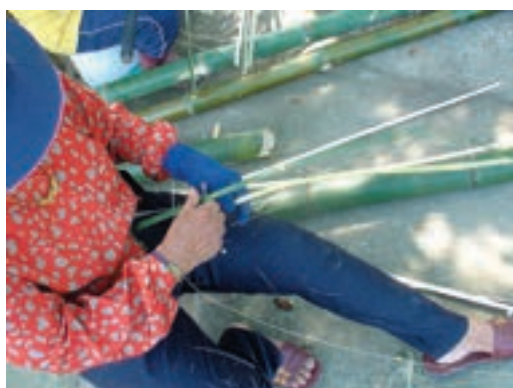
竹條修邊及去內節中隔 Cut the inner part of nodes and smooth the edge of strips.
